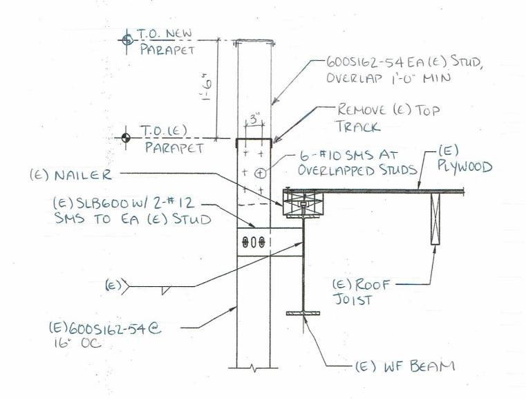
(SK-1) EXTENDED PARAPET DETAIL
