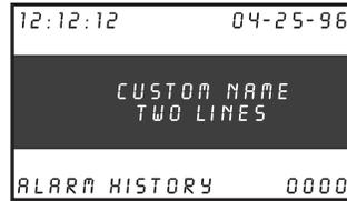
In the center of the 3-LCD is the Liquid Crystal Display. In the normal condition the date and time plus a definable system title display on the LCD. The last line of the display gives an alarm history. This total equals the number of times the system has entered the alarm state from the normal state.
