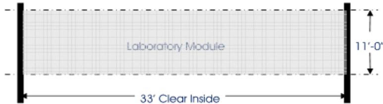
Figure M2 - Laboratory Planning Module
